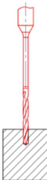
Step 2: Drill CrazyDrill Flex is perfectly guided. Initial position for precise deep hole drilling.
